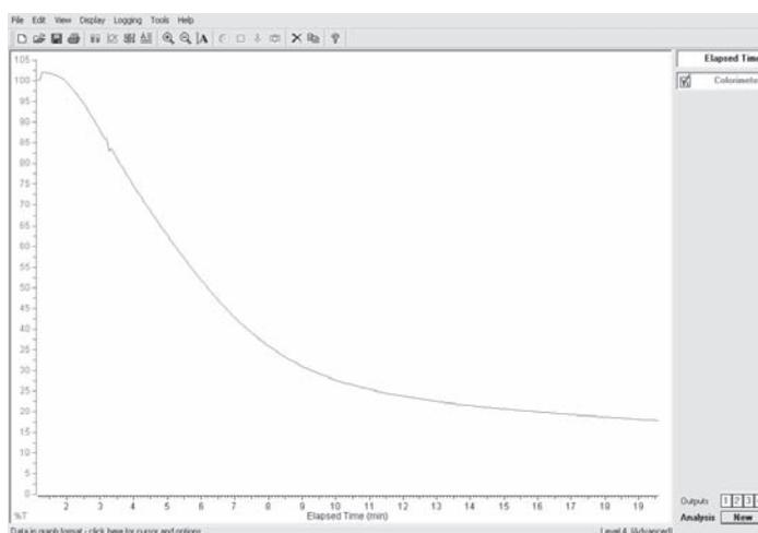
The reaction time can be obtained from the graph from where the plot starts to fall to where the plot levels off again. (The above graph has been zoomed in to show the time of the reaction)
