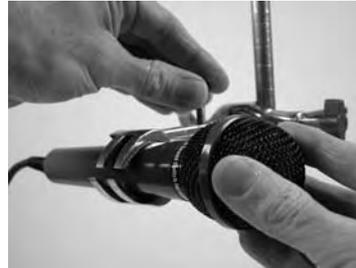
Connect a sound switch to each input on Time Machine. Position the clamp stands so that input 'A' has the first sound switch to receive sound.
