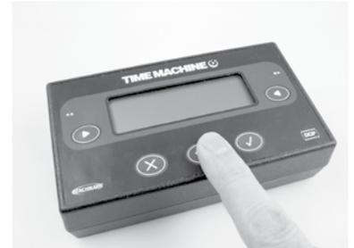
Connect a USB cable to Time Machine, then connect into a suitable USB socket on your computer.
