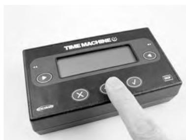
Produce a sound by tapping a wooden block with another hard object. The speed from A to B will be displayed along with the average .
