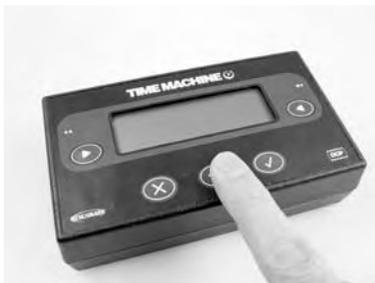
Select 'Lap Timer' from the menu and start running. Time Machine will start recording when the pressure mat is first depressed.
