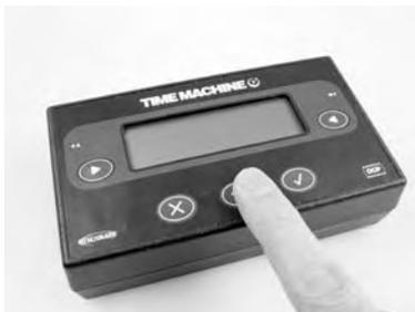
Switch on Time Machine and select 'Time'. Then select 'Time from A to B'.
