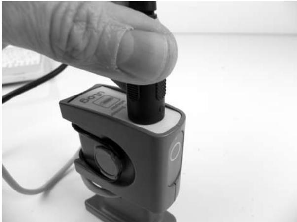
2. Place a small amount of modelling clay to the bottom of the mass and place the mass on the force sensor as shown.
