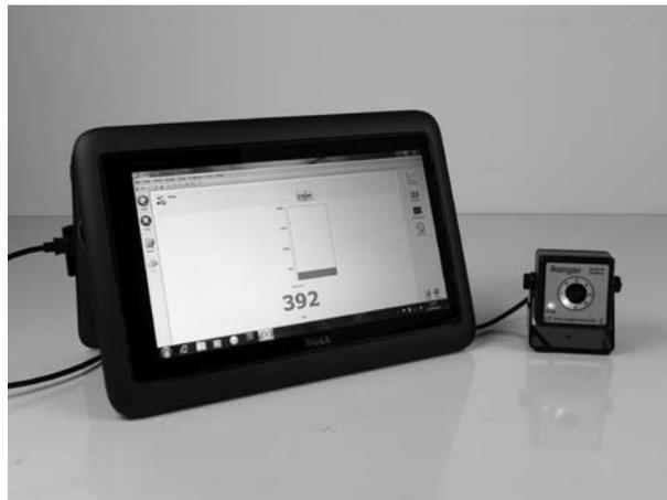
2. Position the uLog Ranger a set distance from a solid object such as a wall. (The larger the target the better).
