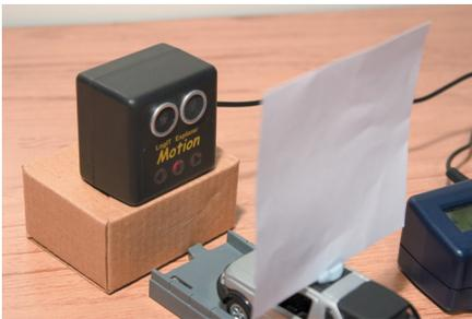
1. Put the ramp in front of the Motion sensor at a small angle.
