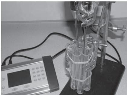
1. Connect the Temperature sensors to the datalogger.
