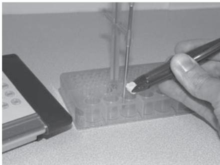
1. Connect the Temperature sensor to the datalogger.
