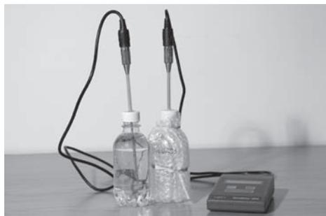
1. Connect the Temperature sensors to the datalogger.
